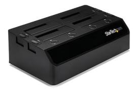
The SDOCK4U33 four-bay 2.5/3.5" SATA HDD / SSD docking station lets you dock and swap four drives from your desktop or laptop computer simultaneously, using a single USB port.
